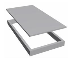
Drill pilots through the plywood into the box frame about every **6 in**. Placement will matter for aesthetic reasons if you are not planning on painting eventually. Also make sure not to drill into the horizontal screws holding the box frame together.
