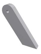
Granted the circular pivots are structurally and aesthetically beneficial, but they do take a certain degree of craftsmanship to achieve. Fortunately, any contour will also work so long as the cut-lines are inside of a bounding radius of 1.75 in. A common alternative to
