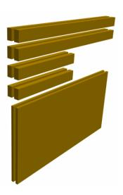
Gather the **48 in** and **21 in** segments and plywood sheets. If framing or box clamps are available to you, now would be a good time to grab them. Mock up or "dry fit" the pieces together on level ground. The longer segments should sandwhich the shorter ones between them.
